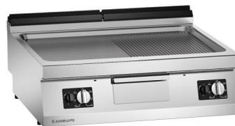
Available only for countries outside the European Community. Griddle made of AISI 304 stainless steel, 20/10 mm thickness top. Satin finished Fe510D steel cooking plate. Delivered with: plate plug. Heating by two independent burner groups controlled by modulating thermostat valve. Working temperature (min-max): 130-320°C.
